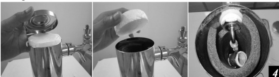
4. Make sure the air hose closes to the top of beer tower at all times, to keep the beer faucet cold.
