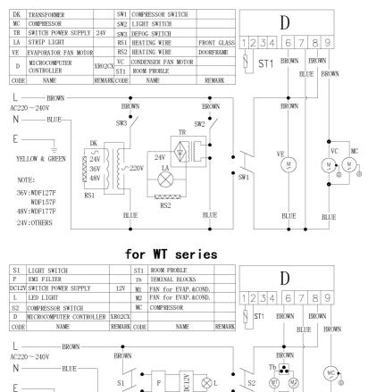
Note: the part in dotted line box is not applicable to some types. Please refer to the real object for the wiring circuit.
