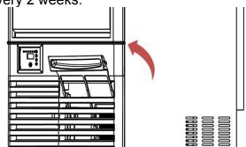
⚠ Note: Be careful when doing the condenser cleaning as the edges of the fins are sharp.
